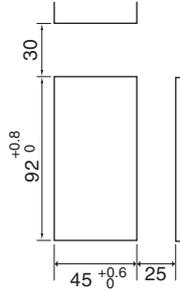
(Panel thickness must be between 1 to 10mm)
