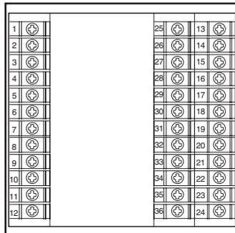
• Use a solderless terminal for screw size M3X6.
