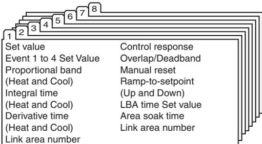
Up to 16-segment ramp/soak control is available by using the memory area function (ramp-to-set point UP and DOWN, soak time, link area number).
